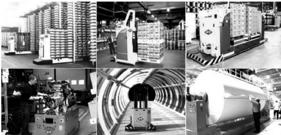
Fig. 1.22. Examples of AGVs for material handling (courtesy of E&K Automation GmbH)
