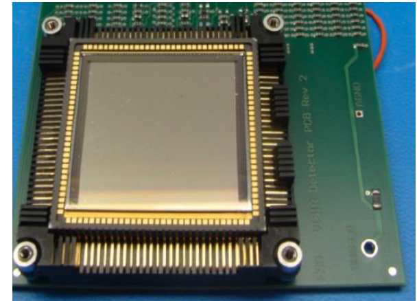
1024x1024 Si:As AQUARIUS Raytheon Vision Systems mid-IR sensor for VLT
