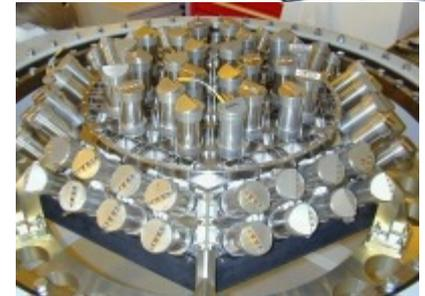
SPI (Spectrometer on INTEGRAL) 20 keV - 8 MeV
