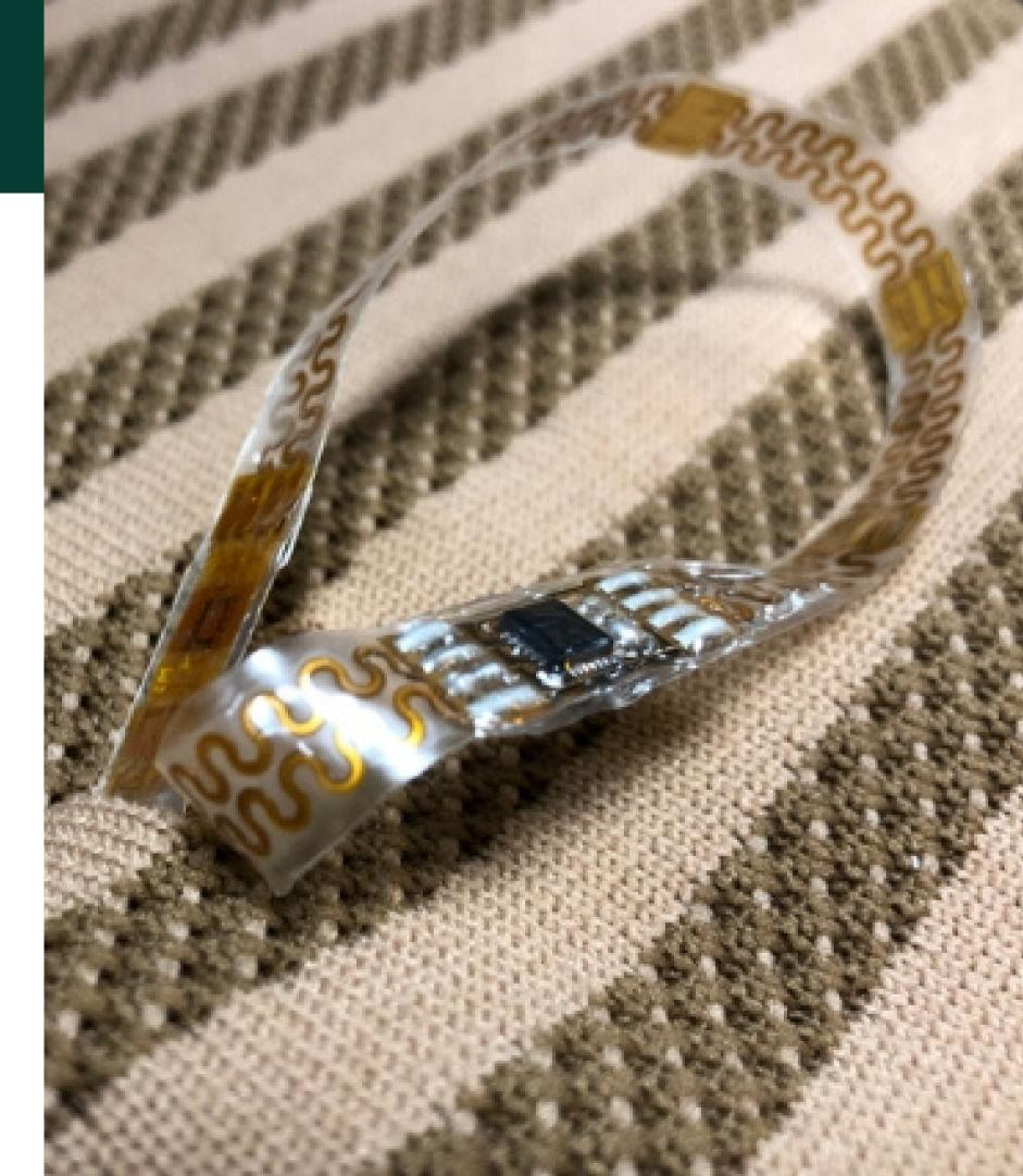
One of the main aspect of wearable technology is stretchability: high performance and elastic mechanical response are an ideal choice for the next generation of healthcare applications.
