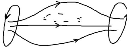
$$\sin \theta_{or} = \left( \frac{v_{\perp 0}}{v_0} \right)^{1/2}$$
