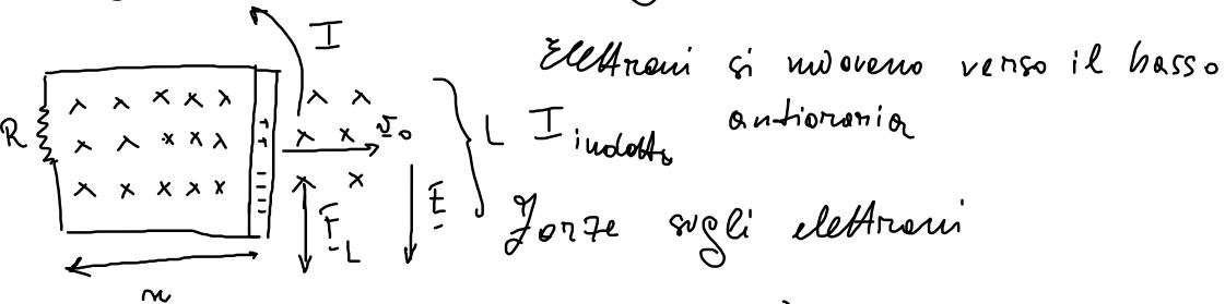
$$-e(\underline{v} \times \underline{B}) - e\underline{E} = \underline{0} \Rightarrow \underline{E} = -(\underline{v}_0 \times \underline{B})$$
