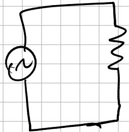
$$\Delta V(t) = \Delta V_{\text{fraz}} \cdot \sin(\omega t)$$
