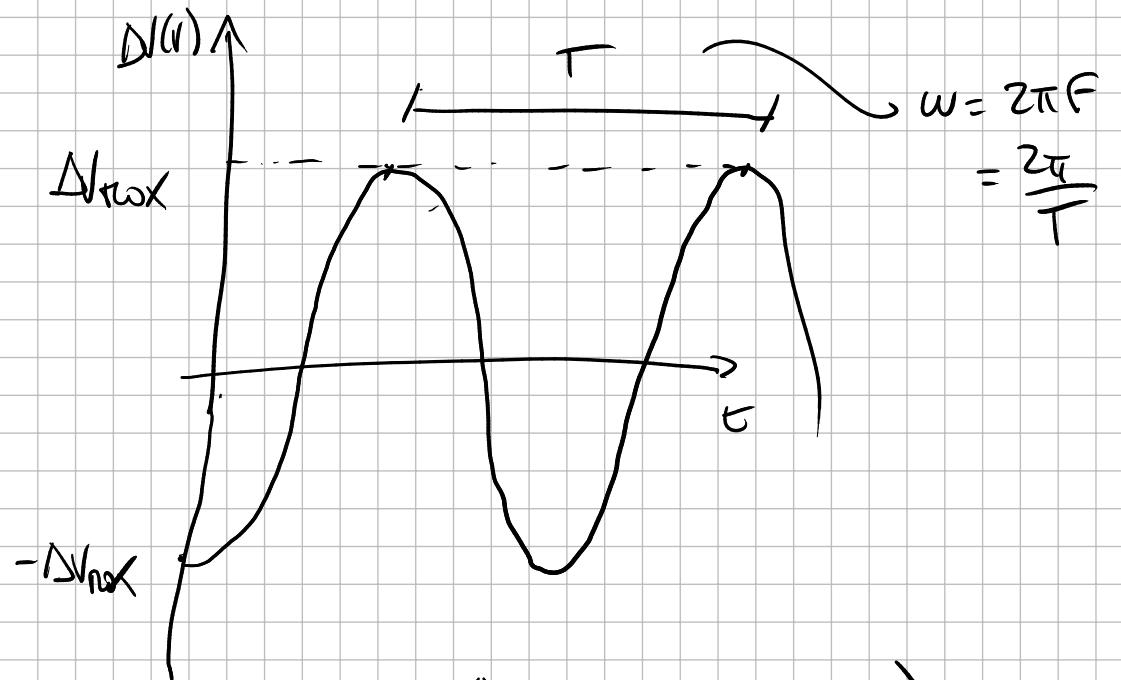
$$\Delta V(t) = \Delta V_{\text{max}} \cdot \sin(\omega t)$$
