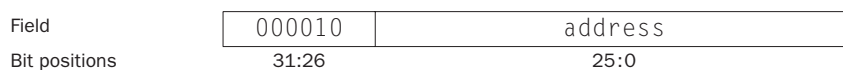
FIGURE 5.23 Instruction format for the jump instruction (opcode = 2). The destination address for a jump instruction is formed by concatenating the upper 4 bits of the current PC + 4 to the 26-bit address field in the jump instruction and adding 00 as the 2 low-order bits.
