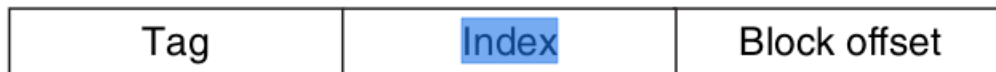
FIGURE 5.17 The three portions of an address in a set-associative or direct-mapped cache. The index is used to select the set, then the tag is used to choose the block by comparison with the blocks in the selected set. The block offset is the address of the desired data within the block.
