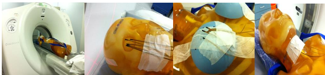
Figure 9.4 – Examples of use of anthropomorphic phantom to assess organ dose in CT (courtesy Rob Loader).
