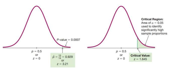
If the XSORT method would not be effective, a sample result equal to or more extreme (in the tail of the distribution) than that observed in the sample (13 girls out of 14 births) would occur 7 times out of 10000.
