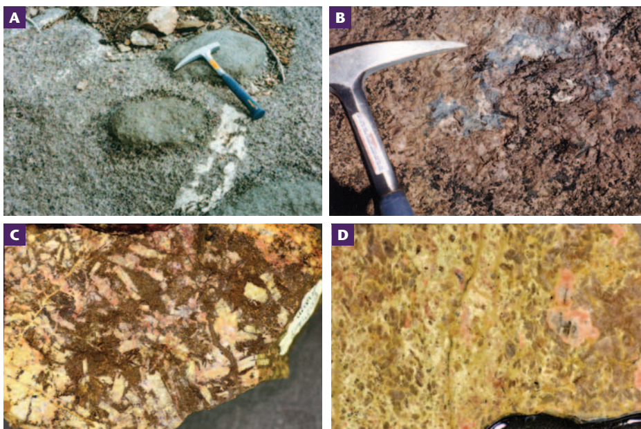
FIGURE 2 Mountain Pass rocks. (A) Xenolith of shonkinite in amphibole syenite, providing a sequence of emplacement. (B) Asbestiform magnesio-riebeckite in amphibole syenite. (C) “Birthday Claim” tabular bastnäsite in a ferruginous dolomite matrix (field of view = 8 cm). (D) Bastnäsite-rich barite sövite in plain light (field of view = 3.6 cm)
