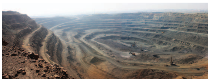
FIGURE 5 The main ore body at Bayan Obo, mined from a large open pit
