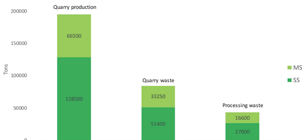
Fig. 3. Quarry production, quarry and processing waste for [SS] and [MS] in t/yr.
