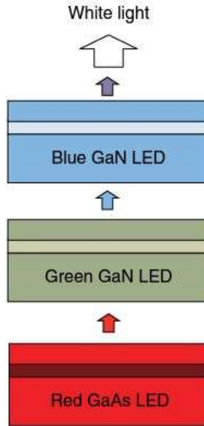
Figure 7.3 Two ways to produce white light from GaN LEDs (DenBaars, 2008).
