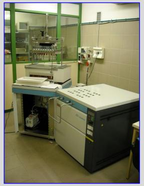
Thermo Finnigan Delta Plus Mas Spectrometer with HDO automatic device.
