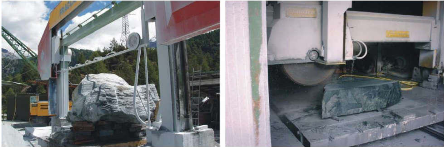
Fig. 2. Serpentinite processing activities, diamond wire squaring off of blocks (on the left) and diamond disk cutting (on the right).
