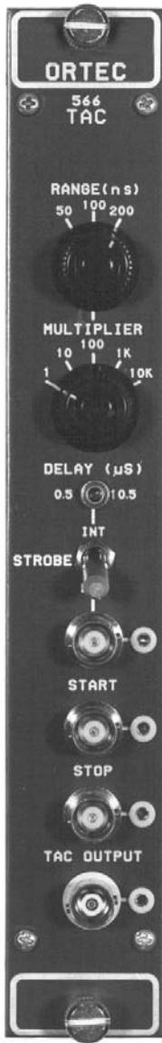
The ORTEC Model 566 Time-to-Amplitude Converter (TAC) measures the time interval between pulses to its start and stop inputs and generates an analog output pulse proportional to the measured time. Timing experiments requiring time ranges from 10 ns to 2 ms may be performed, giving the experimenter flexibility in analyzing random nuclear events that occur within a selected time range. Time ranges from 50 ns to 2 ms are provided via the front-panel controls.
