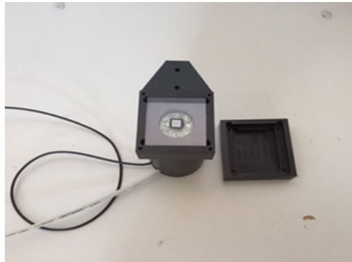
Figure 20: Plastic Scintillator read out with a SiPM
