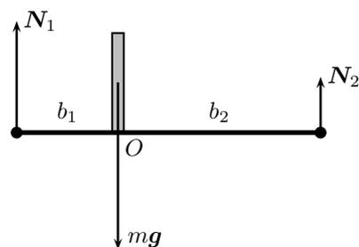
$$\begin{cases} N_1 + N_2 = mg \\ N_1 b_1 = N_2 b_2 \end{cases} \quad \longrightarrow \quad \begin{cases} N_1 = \frac{b_2}{b_1 + b_2} mg = \frac{2}{3} mg = 1.60 \text{ N} \\ N_2 = \frac{b_1}{b_1 + b_2} mg = \frac{1}{3} mg = 0.80 \text{ N} \end{cases} .$$
