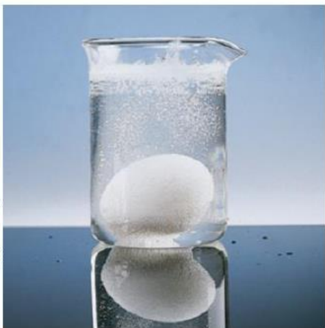
(a) A fresh egg is placed in dilute acetic acid. The acid reacts with the \text{CaCO}_3 of the shell but leaves the egg membrane intact.
