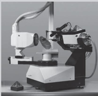
Figure 2.6 A modern CCD diffractometer. Note the circular area detector on the left, which acts as a very sensitive electronic, reusable equivalent of photographic film, allowing many data points to be collected simultaneously. (Photograph courtesy of Nonius.).
